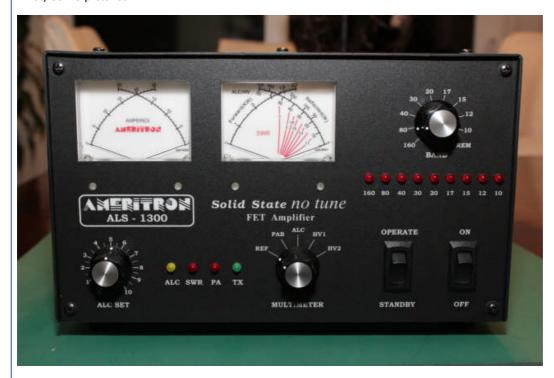
The face of the amplifier is large and the controls are easy to read and use. Once hooked up, the amp is literally a turn-on-and-play deal. One note, you can't just leave the Standby switch in the Operate position and turn it on. You must actively switch the Standby switch to Operate; if it was already in Operate when you turn it on, you must toggle it. This is actually a pretty good minor insurance feature. Then just switch it to the band you want to use and you're ready to go.
