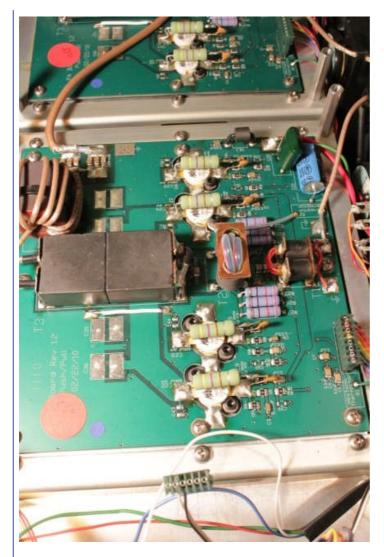
The PA's are run in parallel and each use 4 MRF-150 MOSFETs. I'm no amplifier/circuit design guru, but when I compare schematics it appears to me that the design used is based off of Helge Granberg's Motorola EB104 application which can be found here: <u>High Power Solid State Amplifier</u>.
