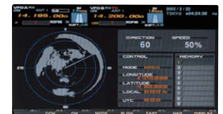
■ Antenna Bearing Indication using Great Circle Map
