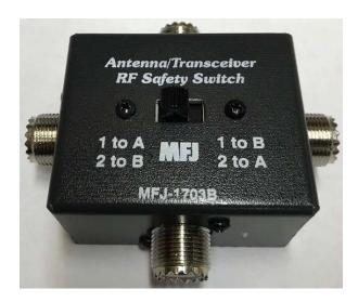
The MFJ-1703B is an antenna-to-transceiver safety switch designed to help protect your radios by ensuring both radios are always connected to an antenna. You can also connect a dummy load and easily switch between the antenna and dummy load.
