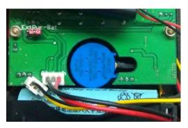
MFJ-266C is off. For charging the position of the EXT PWR-BAT jumper does not matter. It will charge in either position.
