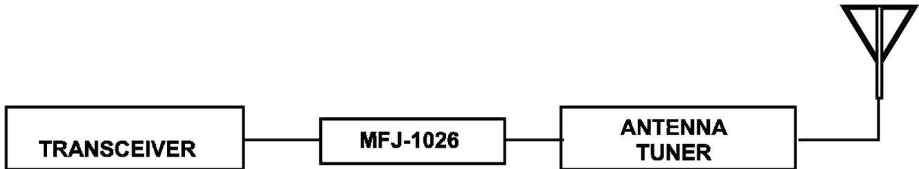
When using an amplifier install the MFJ-1026 between the transceiver and the amplifier input. NEVER install the MFJ-1026 on the output of either an amplifier or antenna tuner!
