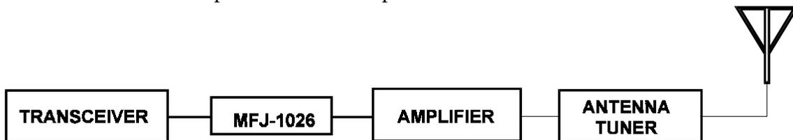
**NEVER** install the MFJ-1026 after an antenna tuner or an amplifier, due to the RF power and voltage handling limits of the unit. The RF power handling limit of the MFJ-1026 is approximately 100 watts.
