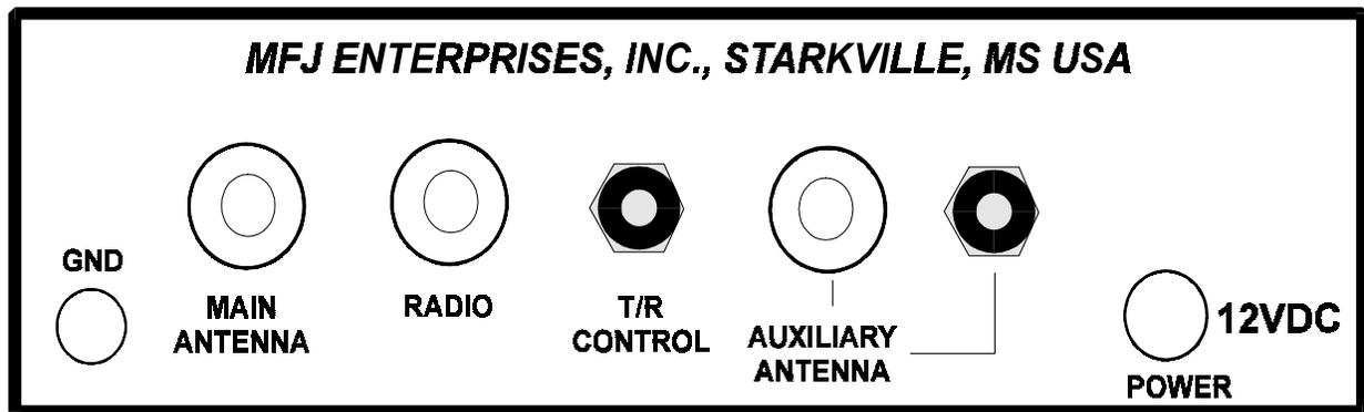
**GND:** This connection is used to connect the MFJ-1026 to the station ground buss. Always use a short ground wire when making this connection. Always try to use solid copper wire (not braided wire) when making a ground connection. Woven or braided wire has higher RF resistance than solid conductors.
