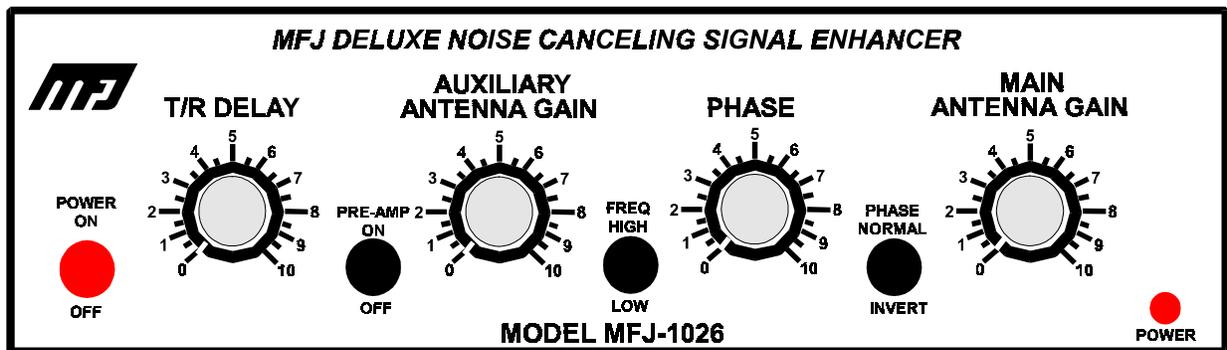
**POWER ON/OFF:** This switch turns the main power off and on. In the OFF (out) position, the MFJ-1026 is bypassed. The RADIO and MAIN ANTENNA connectors have a direct connection between each other whenever power is removed or this switch is turned off.
