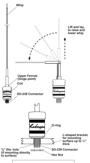
Tech Tip: This antenna will read "open circuit" when tested with an ohm meter or continuity tester.
