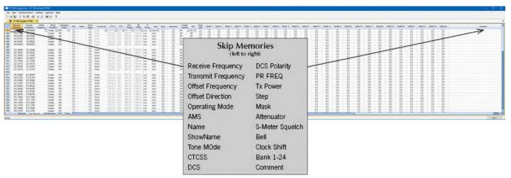
These frequencies are skipped during VFO scanning. These channels can be used for additional regular memory storage if you don't use VFO scanning.
