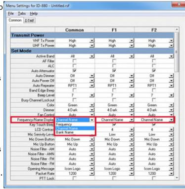
the function of a channel. (Notice the frequency is the same for ALL these channels although they each do something different on the D-STAR network.) Make the Name something you understand.
