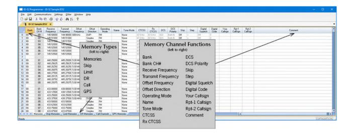
The WCS-D52 Radio Programming Software is designed to make it easier to program your radio. Details of memory channels and other set menu options of your radio are in the program to access and study at your pace. No more "function key frustration" from trying to set options from the face of the radio.
