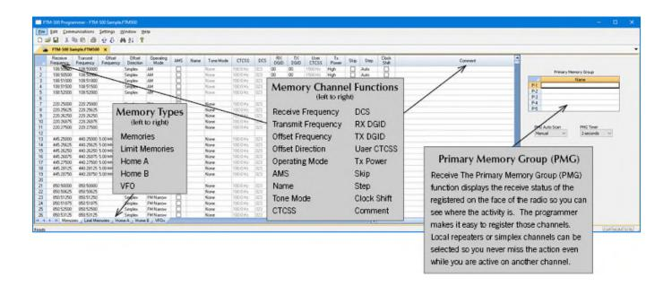
The YPS-M500 Radio Programming Software is designed to make it easier to program your radio. Details of memory channels and other set menu options of your radio are in the program to access and study at your pace. No more "function key frustration" from trying to set options from the face of the radio.
