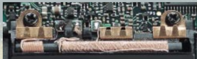
Internal ferrite bar antenna
