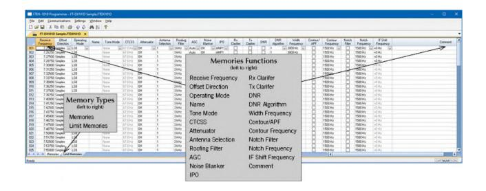
The YPS-DX101D Radio Programming Software is designed to make it easier to program your radio. Details of memory channels and other set menu options of your radio are in the program to access and study at your pace. No more "function key frustration" from trying to set options from the face of the radio.
