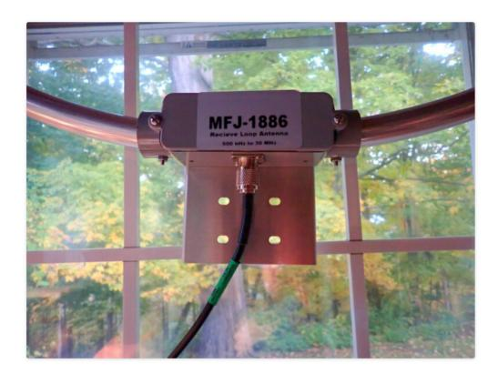
Setting up the 1886 loop is super easy. First, attach a length of coax to bottom of the amplifier box. (The 1886 uses SO-239 connectors.) Attach that coax to the top of the Bias Tee. The Bias Tee supplies power to the amplifier mounted on the loop using the coax and without introducing noise. Run another piece of coax from the bottom of the Bias Tee to the receiver, and, finally, plug the power supply into the Bias Tee and the house power where you are using the antenna.
