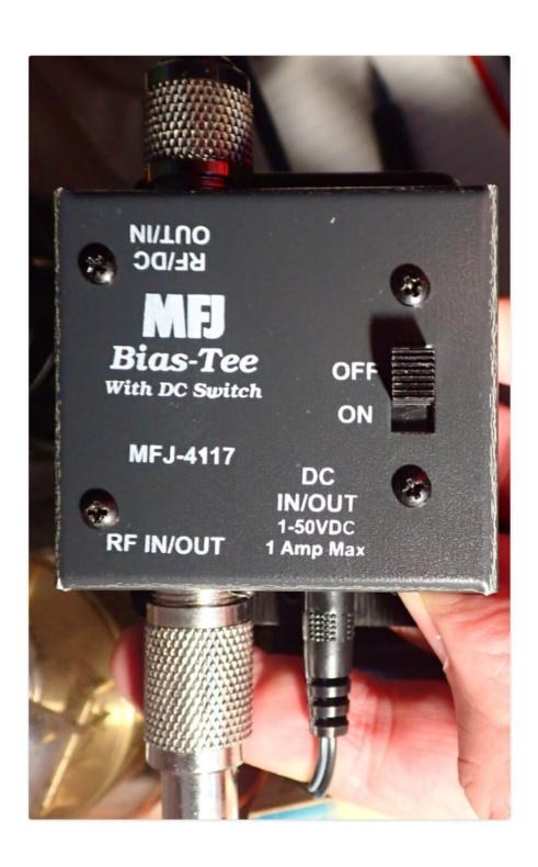
Operating the 1886 is even easier. To hear the signal from the loop *without* amplification, leave the Bias Tee switch in the OFF position. To hear the signal *with* amplification, just slide the switch to the ON position. That's all there is to it. There are no fussy adjustments to make.
