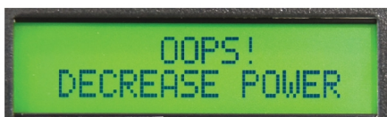
Figure 6 — If you exceed 1,500 W output for more than a second or two, the MFJ-828 alerts you in several ways as described in the text. (Yes, this test was done using a dummy load.)
