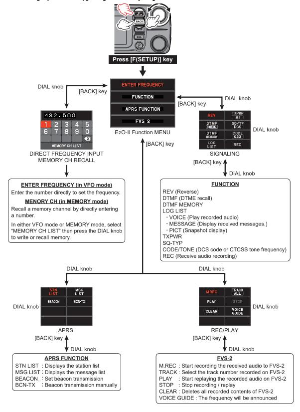
■ To set other functions, call up the menu screen by pressing and holding the [F(SETUP)] key.
