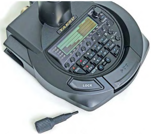
Figure 13 — The Yaesu M-1 microphone top view of the EQ and other adjustments.
