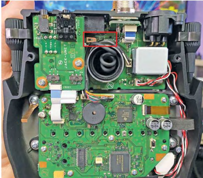
Figure 11 — The Yaesu M-1 internal DCIN switch to select an external power source from the transceiver.
