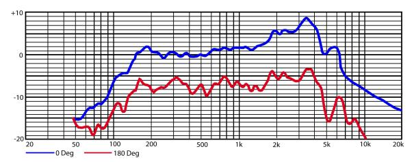
The HC-6 dynamic element, employed in the PSE-6, begins its low-frequency roll-off at about 180 Hz, and it begins to rise at about 1500 Hz; the peak in response, at 3500 Hz, is approximately 9 dB, with the enhancement being between 5 and 6 dB between 2000 and 3000 Hz (the upper end of a typical SSB bandwidth).
