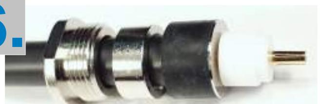
Slide center pin (Pin 1, 2,8mm Ø) on center conductor and solder carefully. Then attach teflon isolator.
