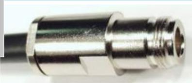
Slide the prepared cable end into the connector housing until stop. Tighten smoothly with two wrenches 17 mm and 18 mm so that there is still a small gap visible between the nut and the connector housing.
