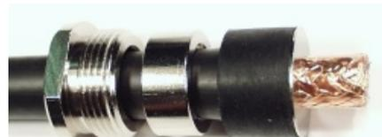
Bend copper braid at 90 degrees to cable body. Push in contact ferrule between copper foil and braid until stop. Trim braid even to rim of ferrule. Slide rubber gasket down to the contact ferrule.
