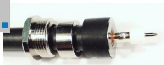
Slide center pin (Pin 1, 2,8mm Ø) on center conductor and solder carefully. Then attach teflon isolator.
