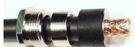
Bend copper braid at 90 degrees to cable body. Push in contact ferrule between copper foil and braid until stop. Trim braid even to rim of ferrule. Slide rubber gasket down to the contact ferrule.
