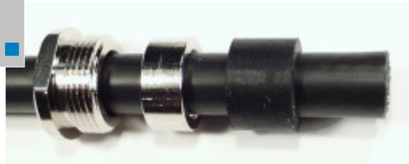
Slip the nut, the pressure ring and the rubber gasket over the cable end.
