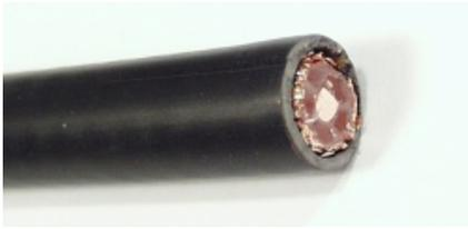
Cut the cable end perpendicularly
