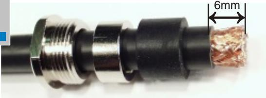
Remove 6 mm of the PVC sheath from the end of the cable with a knife.
