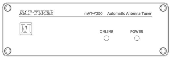
**ONLINE:** Status indication. Lights up to indicate that the tuner is online, off-indicates that the tuner is bypass.
