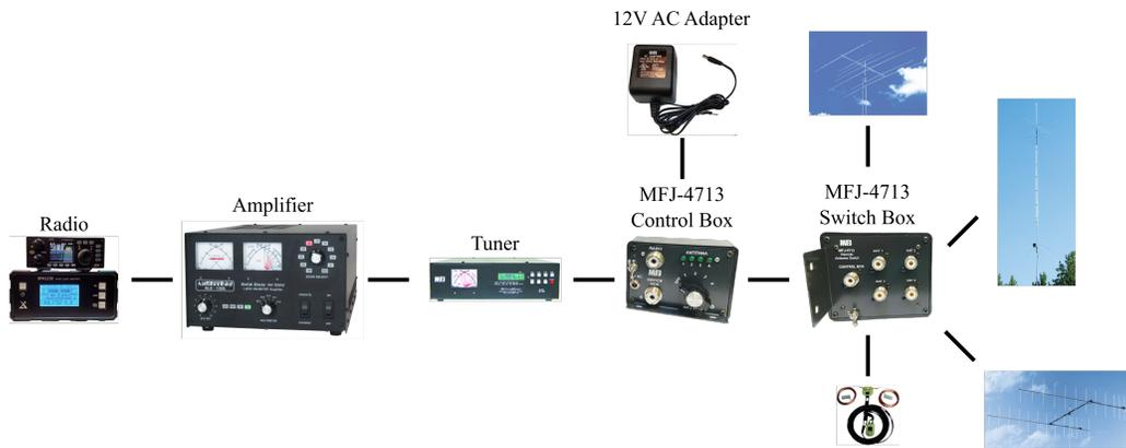
Figure 4: MFJ-4713 Station Setup
