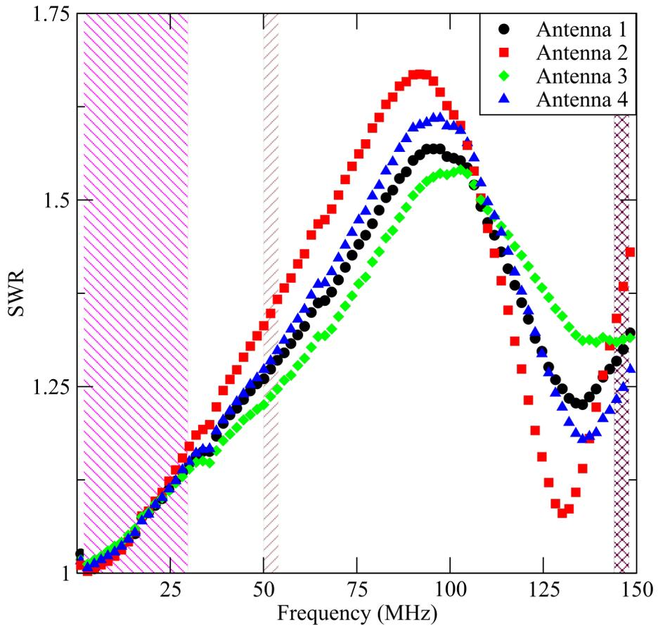
Figure 2: SWR plot of each antenna port. HF and VHF frequencies are highlighted.
