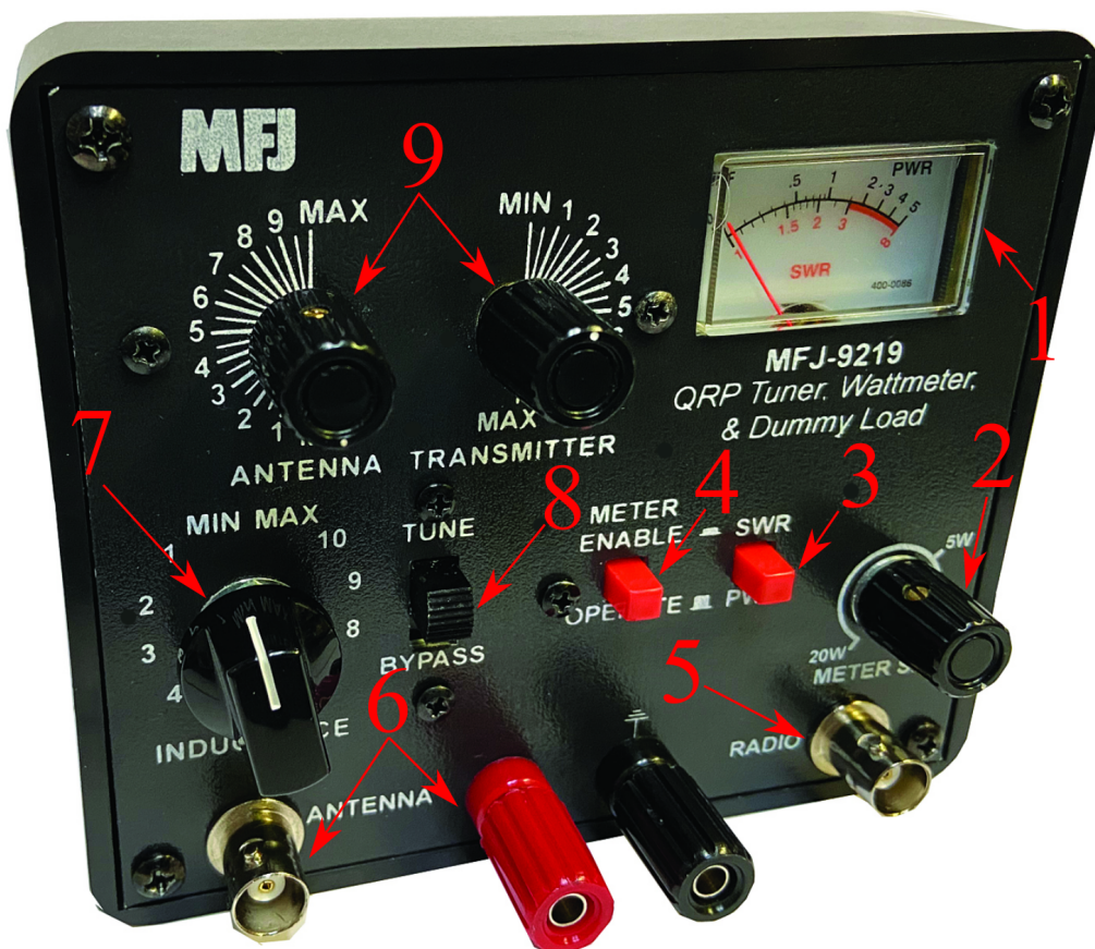
Figure 5: MFJ-9219 Controls. 1.) Multipurpose Meter, 2.) SWR Circuit BYPASS Switch, 3.) SWR/PWR Switch, 4.) METER SENSITIVITY Knob, 5.) RADIO Connection, 6.) ANTENNA Connection, 7.) INDUCTANCE Control, 8.) Tuner BYPASS Control, 9.) ANTENNA and TRANSMITTER Controls
