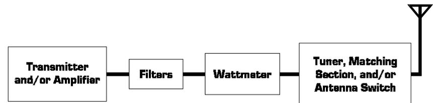
If you want to measure the power capability of a transmitter/amplifier or to recalibrate the MFJ-862 you should connect a quality dummy load (50 ohms) that is designed for VHF/UHF to the antenna jack.
