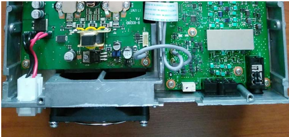
After removing Tuner Jack with Cable Assembly
