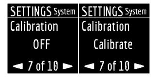
The OFF item turns off the calibration, and the Calibrate item starts the calibration process.
