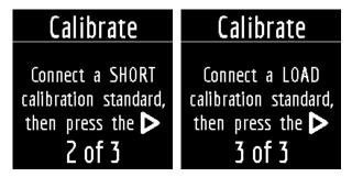
Remember to prepare the calibration kit in advance! During the calibration process, the analyzer screen looks something like this:
