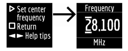
The keys select the cursor position to change units, tens, hundreds, thousands of kilohertz, and the setting the measurement bandwidth by pressing the keys.
