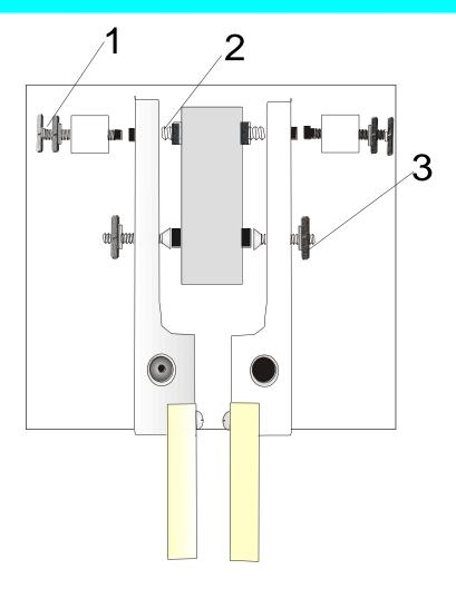
**CONTACT - SPACING:** Spacing between the lever arm contacts and the contact post set screws is realized by adjusting the contact set screw to increase or decrease the distance. (1)
