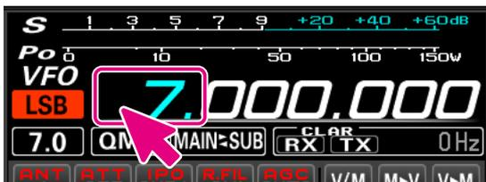
2. In this state, turning the mouse wheel will change the frequency in 1MHz steps.
