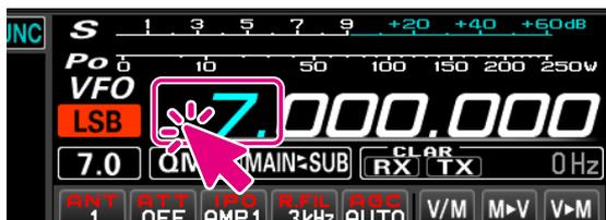
**Wheel:** Move frequency Up / down at 1MHz
