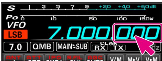
2. In this state, turning the mouse wheel will change the frequency in the set “**TUNING**” step.
